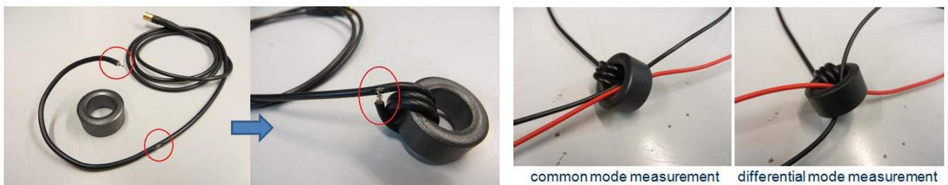
Figure 8. High Frequency Current Probe Construction
