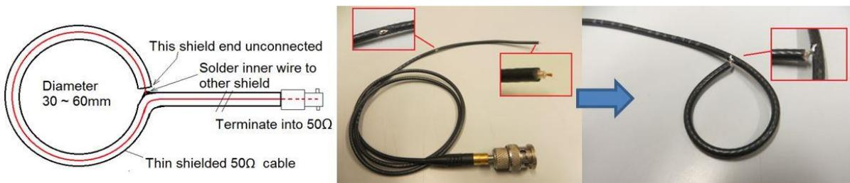
Figure 7. High Frequency Current Loop
